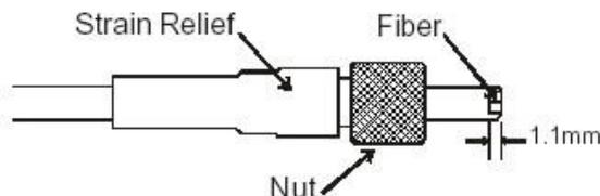
Figure 1: High Power SMA Connector Design
