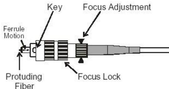
Figure 2: High Power Adjustable Focus FC Connector Design
